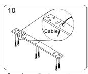
Once the position is correct, use the screws to permanently mount the mounting plate, And drill the cable access hole.
