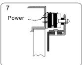
Turn on the power of EM-Lock, and let the armature plate bonds to the EM-lock. Adjust the position between the Z bracket and the door frame.
