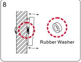
This will allow the armature plate to pivot slightly around the armature screw in order to compensate for door misalignment.
