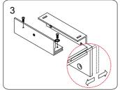
Assemble the Z bracket, and make sure that the Z bracket is adjustable.
