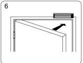
Close the door. Measure the correct position by bringing the armature plate close to the contact surface of the electromagnetic lock.
