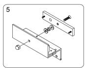
Put one rubber washer between armature plate and the Z bracket, and place them over the 8mm armature screw.
