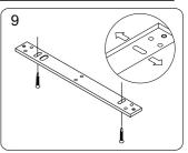
Screw the two self-tapping screws in the slotted holes of the mounting plate and adjust the position of the mounting plate so that it and the armature plate from a 90-degree
