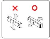
During the installation procedure, it is important to make sure that the working direction of the armature plate has to be facing toward the contact surface of the electromagnetic lock intend to have the maximum holding force.
