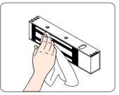
Apply a light coat of a silicon lubricant to prevent rust. Wipe away the excess.
