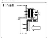
Once the position is correct, use the screws to permanently mount the Z bracket on the door frame. This should be the last step.
