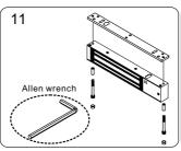
Use the Allen wrench to screw the Fixing screws and Brass Sleeves through the bottom of the electromagnet into the mounting
