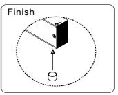
Insert the anti-tamper caps into the mounting screw access holes. This should be the last step, as once the tamper caps are in place, they will be difficult to remove.
