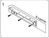
Find a mounting location on the door frame for the L bracket. Make sure that the door is still closeable.
